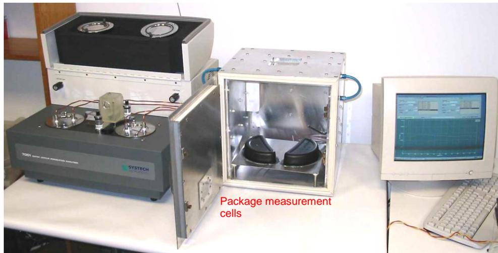
Figure 4 : Systech 7001 Water permeability measurement
