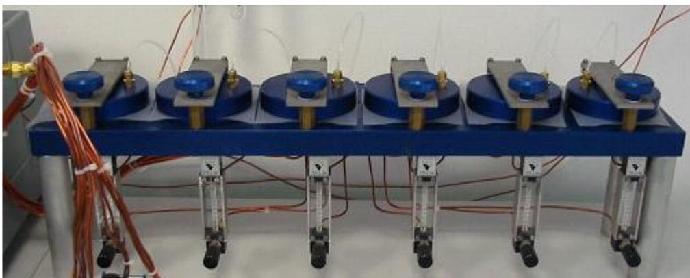
Figure 3 : Weak permeability film device
