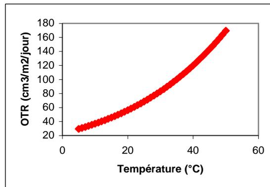
Figure 5 : Variation of a 23µm PET film permeability with temperature
