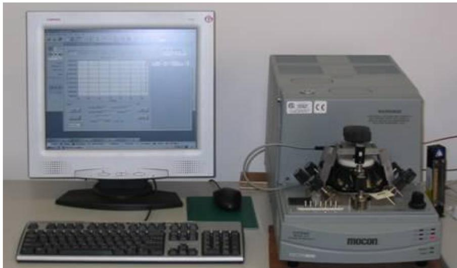
*Figure 1 : Mocon OxTran 2.61 (oxygen permeability measurement)*
